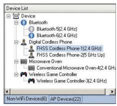
Figure 4: Detect and classify interfering sources
