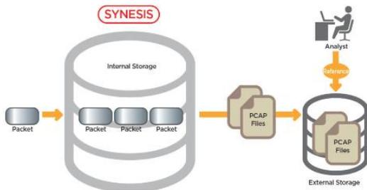
SYNESIS is a capture appliance compatible with 10M/100M/1G/10G/100G networks that can capture traffic at wire speed without data loss. A backup function allows saving to PCAP files automatically while capturing. The storage destination can either be a local or remote file system.
